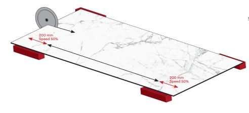
Make sure the slabs are fully supported on the cutting bench and that there is no waste on either the slab or the disc (the disk segments must be honed regularly). The slabs must be secured on the cutting bench with clamps. The use of a material such as Ecorubber (a high density rubber) between the bench and the material is recommended to improve cutting quality.
