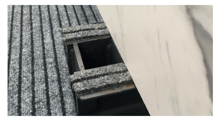
Slabs can be laid one on top of another, although no slabs or parts of slabs must be rested on top of smaller slabs or waste materials; always check that all parts of the slab are resting on something and that there are no gaps. Do not rest stone or quartz material on top of ceramic slabs, especially those which are larger in size and thicker than the ceramic slabs.
