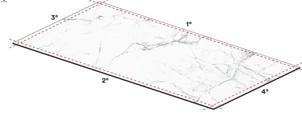
We recommend you cut the slabs with a segmented cutting disc for ceramics. Speed at which the disc is lowered onto the bench 0.1 m/min. Disc recommended for cutting porcelain slabs: we recommend you use an ADI disc (type: MTJ64002) which can be used for both straight and 45° cutting. This tool can be used on different bridge cutters with different technical parameters.
